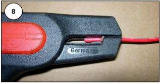
The Wurth pliers are simpler in operation. After placing the cable in the "V" of the bottom ILL 7, squeeze the handles together. The squeezing action brings the jaws together and forces the bottom jaw forward both cutting and pulling the sheath from the cable. See ILL 8 & 9.
