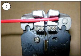
3 Increase the pressure slightly as you continue to squeeze. The stripping jaws will then move indipendantly of the pliers cutting and stripping the end of the wire until with a sharp click both sets of jaws will automatically disengage.
