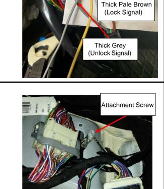
• Run the canopy earth (black with an eye terminal) to the attachment screw.
