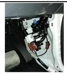
•Unplug all sockets and connect the earth to the existing bolt.
