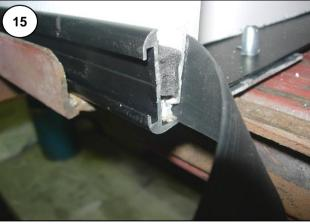
31 Drill 5mm hole through outer rail, panel and shell 10mm from front edge and through the end of the length of vinyl trim. See **Photo 16**.
