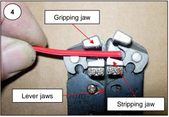
2 Continue squeezing the handles together to engage the gripping and stripping jaws.
