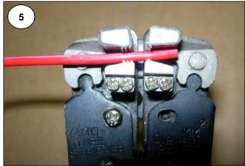
3 Increase the pressure slightly as you continue to squeeze. The stripping jaws will then move independantly of the pliers cutting and stripping the end of the wire until with a sharp click both sets of jaws will automatically disengage.
