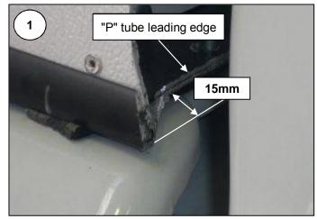
The latch bar supplied gives problems due to the curvature of the tailgate. The door itself is not all that hard to bend once the canopy is on the vehicle but the square cut edges of the latch bar cause it to jam under pressure.
