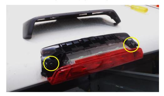
3 Pull out the stop light and unplug from the wiring loom
