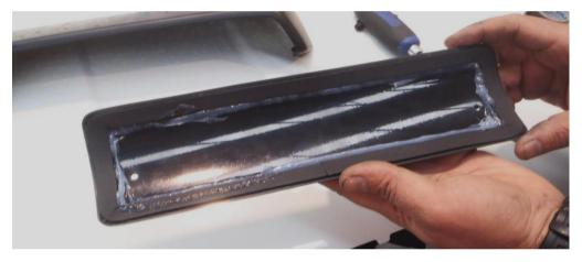
7 Re-use the mounting screws from the stop light to attach the new cover plate. Use them as a guide to line up the cover before sealing against the cabin. Torque by hand until firm but do not over-tighten
