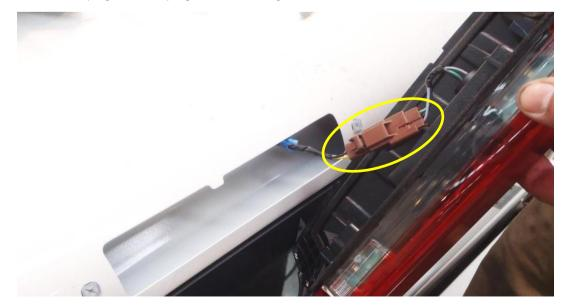
**4** Wrap the plastic connector in electrical tape and secure inside the stop light cavity to ensure it doesn't rattle against the sheet metal
