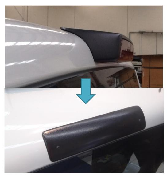
**1** Remove the Black plastic surround of the high mount stop light by gently pulling open the side of the cover and using a flat blade screwdriver to release the plastic clip inside.
