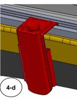
If an over lip liner is fitted holes will need to be cut in the liner to allow the fitment of the six clamps. If an underlip liner is fitted ascertain how stiff the plastic is. If it is too stiff to allow the clamp to be pushed up between it and the metal lip, proceed as follows.
