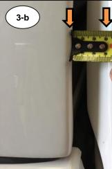
7 There are to be 3 clamps fitted per side. Position as far forward and as far rearward as possible, with the 3rd clamp being fitted central. The clamp underside is fitted around the tub flange while the base rail has adjustability in position via fitment to either of the 3 channels as shown see ILL 4-a,b,c,d
