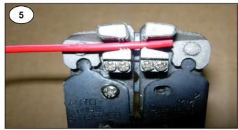
3 Increase the pressure slightly as you continue to squeeze. The stripping jaws will then move independently of the pliers cutting and stripping the end of the wire until with a sharp click both sets of jaws will automatically disengage.
