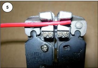
Increase the pressure slightly as you continue to squeeze. The stripping jaws will then move independently of the pliers cutting and stripping the end of the wire until with a sharp click both sets of jaws will automatically disengage.
