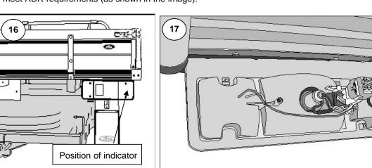
26 The OEM lamps and brackets should now be attached to the underside of the tray rear, ensure that the lenses are fully exposed and the indicator lenses are to the outside. See ILL16.
