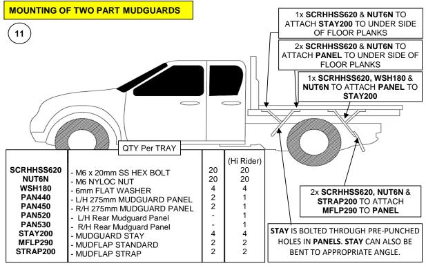
18 Mount the mudguards to the underside of the tray deck by lining up the pre-punched holes in the mudguard with one of the ribs running along the underside of the tray. Attach with 2 of SCRHHSS620 & NUT6N.
