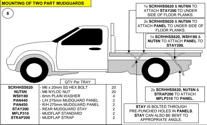
**Note:** Two of the mudguard stays will need to be modified in the following way for the front mudguard panels.
