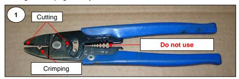
It is a documented fact that the use of these pliers can cause personal injury due to the fact that they are reliant upon holding the cable in one hand while pulling with the pliers with the opposite hand. Any attachments to the gripped end can be pulled into and through the palm of the gripping hand causing injury.
