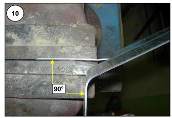
17 Shorten the re-bent end by about 25mm and drill with a 1/4" (6.25mm) drill bit. See ILL 11.
