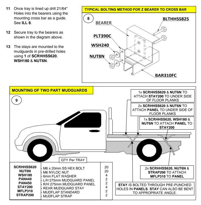
14 Mount the mudguards to the underside of the tray deck by lining up the pre-punched holes in the mudguard with one of the ribs running across the underside of the tray. Drill 1/4" holes and attach with 2 of SCRHHSS620 & NUT6N.
