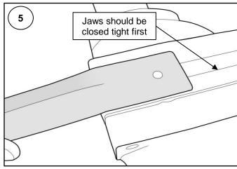
7 Clamp in the vice and bend the flattened end 90° at the mark to make the shape shown in **ILL 6**.
