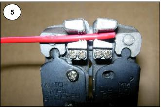
3 Increase the pressure slightly as you continue to squeeze. The stripping jaws will then move indipendantly of the pliers cutting and stripping the end of the wire until with a sharp click both sets of jaws will automatically disengage.
