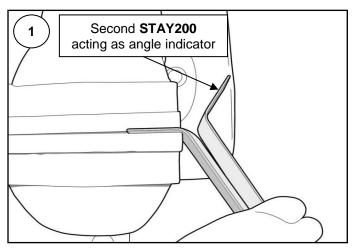
2 Use a second stay as a guide to straighten the bottom end, use the guide stay to achieve about 90° between the two ends. See ILL 2.
