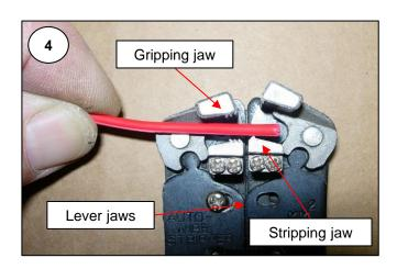
2 Continue squeezing the handles together to engage the gripping and stripping jaws.
