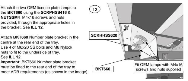
27 The OEM lamps and brackets should now be attached to the underside of the tray rear, ensure that the lenses are fully exposed and the indicator lenses are to the outside.
