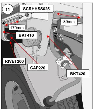
Remove filler cap and fit BKT420 over the filler and position it onto the tray underside. When comfortably positioned clamp to one of the plank flanges and mark holes for fixing. Use a scriber to mark through the filler neck flange holes onto the back of the bracket. See ILL 11.
