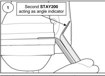
2 Use a second stay as a guide to staighten the bottom end, use the guide stay to achieve about 90° between the two ends. See **ILL 2**.
