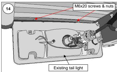
28 All lamps can now be re-connected to the main harness using the existing multi-snap connectors, check for correct operation.
