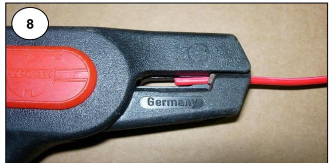
4 The Wurth pliers are simpler in operation. After placing the cable in the "V" of the bottom jaw, ILL 7, squeeze the handles together. The squeezing action brings the jaws together and forces the bottom jaw forward both cutting and pulling the sheath from the cable. See ILL 8 & 9.
