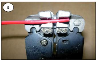
3 Increase the pressure slightly as you continue to squeeze. The stripping jaws will then move indipendantly of the pliers cutting and stripping the end of the wire until with a sharp click both sets of jaws will automatically disengage.
