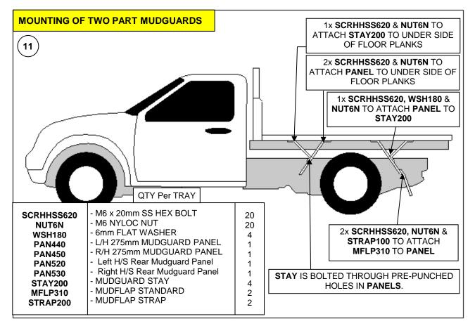
**19** Mount the mudguards to the underside of the tray deck by lining up the pre-punched holes in the mudguard with one of the ribs running along the underside of the tray. Attach with 2 of **SCRHHSS620** & **NUT6N**.
