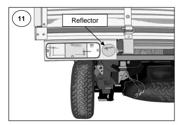
6 If the wiring, complete with multiconnectors, has been cut from the well body lights. Then the LIGHT460's should be connected to it with CON110 in the following manner.
