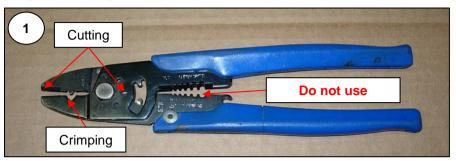
It is a documented fact that the use of these pliers can cause personal injury due to the fact that they are reliant upon holding the cable in one hand while pulling with the pliers with the opposite hand. Any attachments to the gripped end can be pulled into and through the palm of the gripping hand causing injury.
