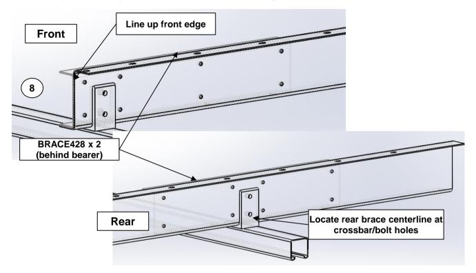
**13** Drill 7mm holes through the bearer and brace at the approximate locations per **ILL 9** below. Note: At least 8 Bolts per brace should be used in each reinforcement
