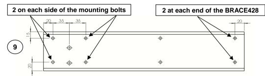
14 Bolt reinforcements tightly to bearer with 8x BLTHHZPF616 and NUT6N per ILL 10 below
