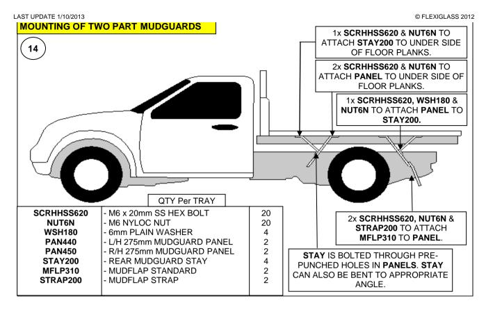
25 Attach the other end of the stay to the underside of the tray using same method but with only one fixing.
