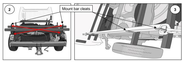
**9** Slide the tray into position with the front end of the main bearers flush with the angle cleat of the cross bar.
