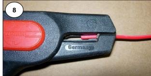
The Wurth pliers are simpler in operation. After placing the cable in the "V" of the bottom jaw, ILL 7, squeeze the handles together. The squeezing action brings the jaws together and forces the bottom jaw forward both cutting and pulling the sheath from the cable. See ILL 8 & 9.
