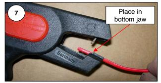
The Wurth pliers are simpler in operation. After placing the cable in the "V" of the bottom jaw, ILL 7, squeeze the handles together. The squeezing action brings the jaws together and forces the bottom jaw forward both cutting and pulling the sheath from the cable. See ILL 8 & 9.
