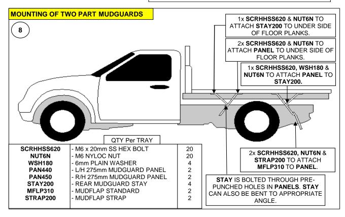
14 Mount the mudguards to the underside of the tray deck by lining up the pre-punched holes in the mudguard with one of the ribs running along the underside of the tray. Drill 1/4" holes and attach with 2 of SCRHHSS620 & NUT6N.
