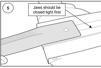
Clamp in the vice and bend the flattened end 90° at the mark to make the shape.
