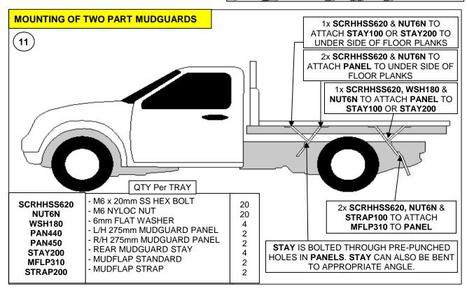
Mount the mudguards to the underside of the tray deck by lining up the pre-punched holes in the mudguard with one of the ribs running along the underside of the tray. Attach with 2 of SCRHHSS620 & NUT6N.
