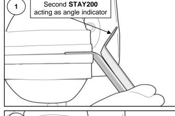
2 Use a second stay as a guide to staighten the bottom end, use the guide stay to achieve about 90° between the two ends. See **ILL 2**.
