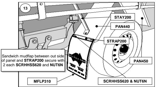
23 Attach both MFLP310 mud flaps to the mudguards using 4 of SCRHHSS620 & NUT6N as well as 2 of STRAP200 as shown in the diagram below.
