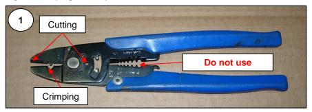
It is a documented fact that the use of these pliers can cause personal injury due to the fact that they are reliant upon holding the cable in one hand while pulling with the pliers with the opposite hand. Any attachments to the gripped end can be pulled into and through the palm of the gripping hand causing injury.
