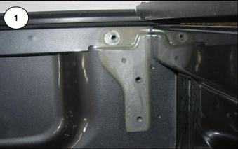
1 Remove the cab-rack using a **#40 Torx driver** and **10mm socket** to release six cup head screws inside the tub and five 10mm hex
