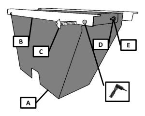
• Fit and fully tighten the **C** (Bolt M6-50), **E** (Washers) & **D** (Nut Nylock N6) to fit **B** (Brackets) brackets to **A** (Slant Water Tank). (The bracket towards outside of the vehicle, must cover the edge of the water tank.)
