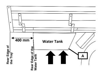
• Leave 400 mm distance between the rear edge of the tray and rear edge of the water tank.
