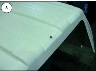
To make positioning of the dust deflector as easy as possible, the canopy can be resting on the ground. This allows the canopy assembler to work over the top and use your finger tips holding the ends of the deflector as a guide to ensure accurate fitting. The tape is quite adhesive so don't apply any pressure until the fit is seen to be good.
