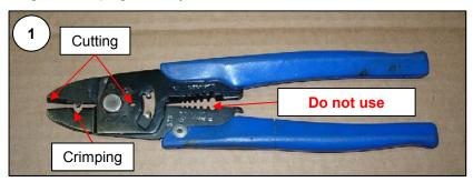
It is a documented fact that the use of these pliers can cause personal injury due to the fact that they are reliant upon holding the cable in one hand while pulling with the pliers with the opposite hand. Any attachments to the gripped end can be pulled into and through the palm of the gripping hand causing injury.
